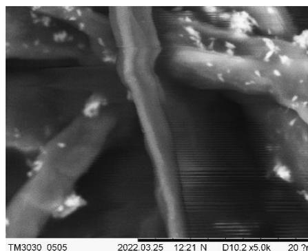
Fig. 3. Close-up of algae fibre on the paper surface, SEM image, magnification 5000x
